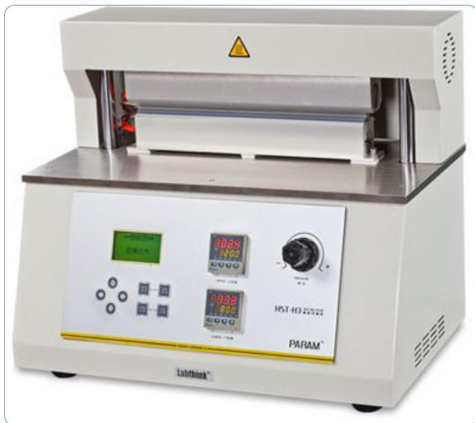
HST-H3 Heat Seal Tester simulates the heat sealing method, and controls temperature, dwell time, and seal pressure for heat sealing of various composite films to guide industrial production. The instrument conforms to multiple national and international standards.
